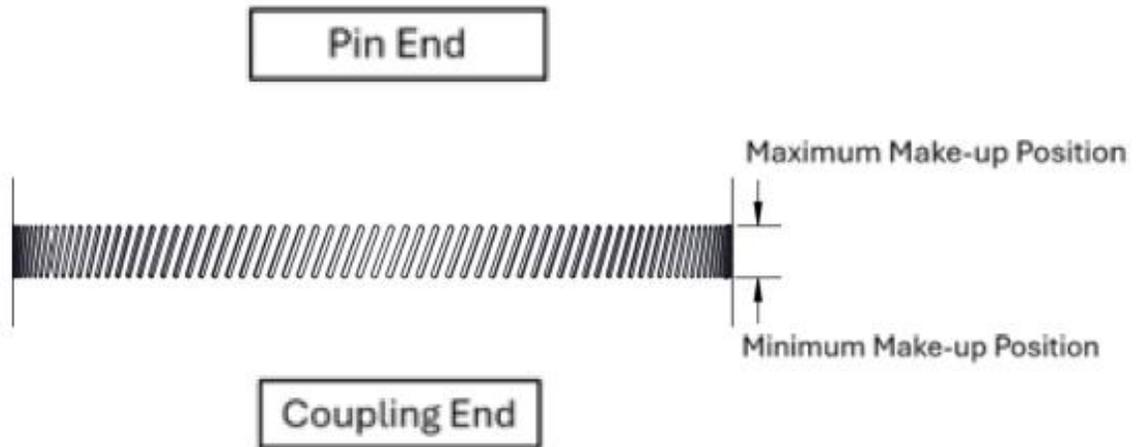
**Figure 10: Knurl Band Tolerance Criteria**
