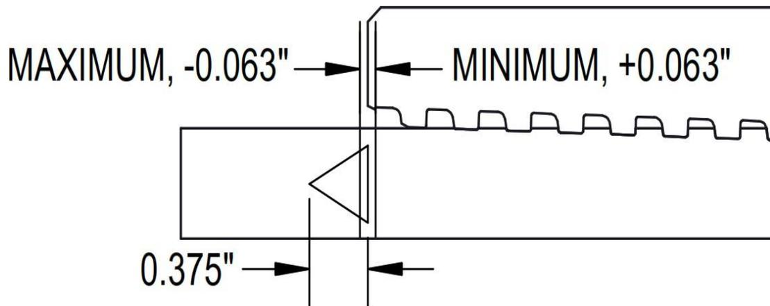
Figure 13: Triangle Stamp Make-Up Tolerance Criteria
