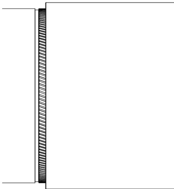
**Figure 11: Knurling Area After Box/Pin Make-Up**
