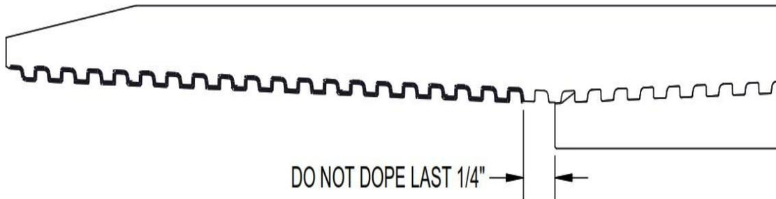
Figure 3: Proper Thread Compound Application Criteria for the Box Ends
