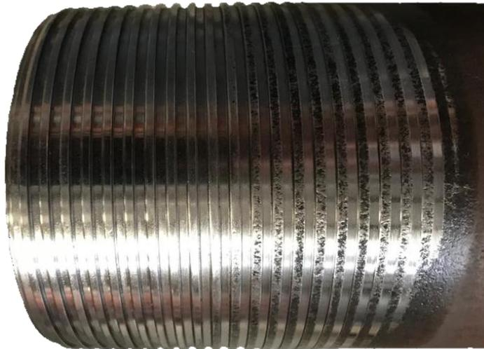
Figure 4: Do NOT Apply Thread Compound to Rattler® Pins
