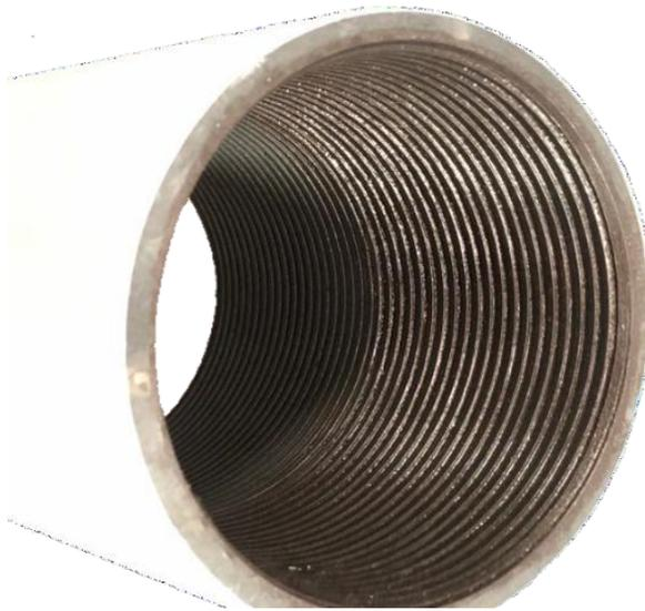
Figure 1: Proper Thread Compound Application Example
