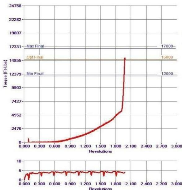
**Figure 7: Example of a Proper Make-up Graph**
