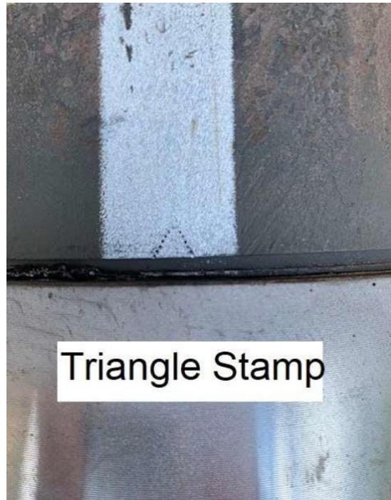
Figure 12: Example of Proper Triangle Stamp Position After Make-Up
