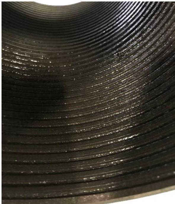
Figure 2: Proper Thread Compound Coverage Example
