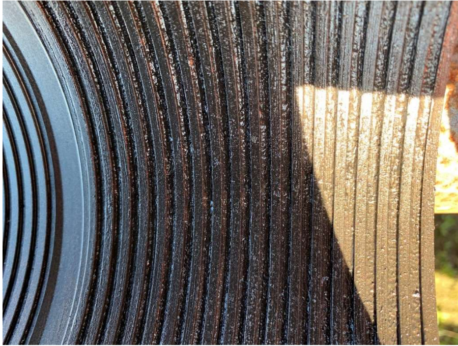
Figure 2: Correct way to apply thread compound to box.
