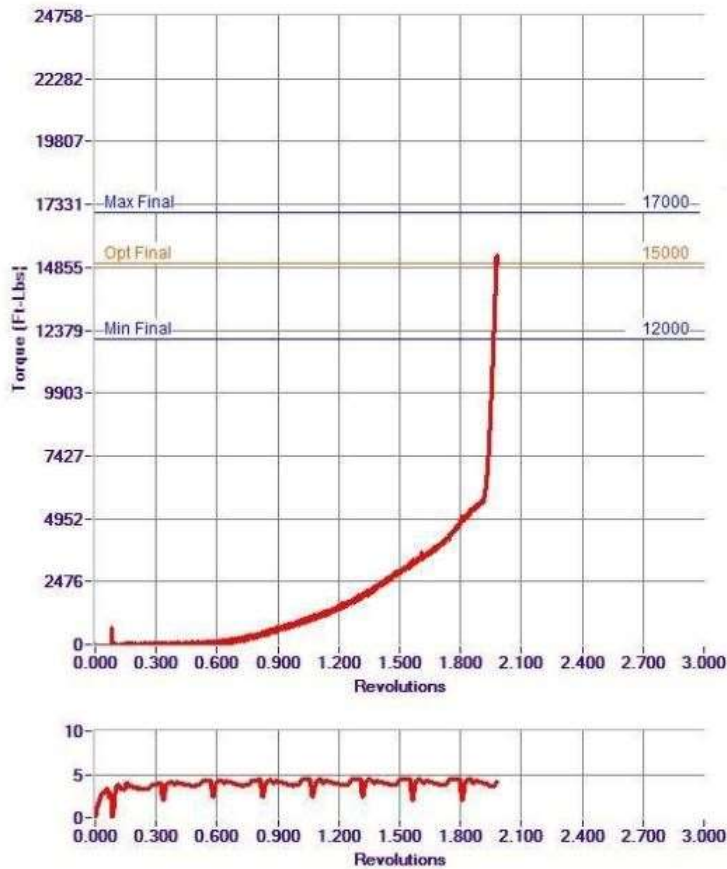
Figure 3: Correct make-up graph.
