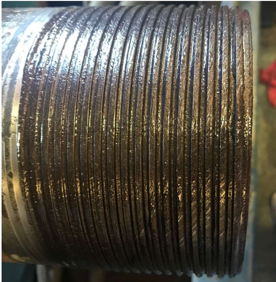
Figure 1: Correct way to apply thread compound to pin.
