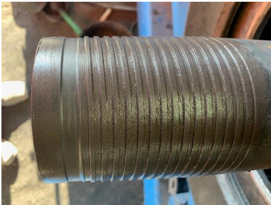
Figure 1: Correct way to apply thread compound.
