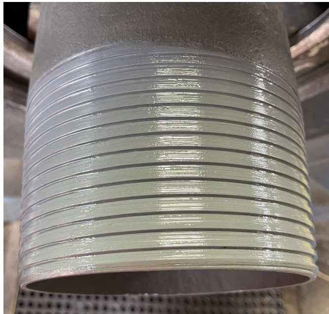
Figure 3: Example of Proper & Acceptable Thread Compound Application of the Pin Connection
