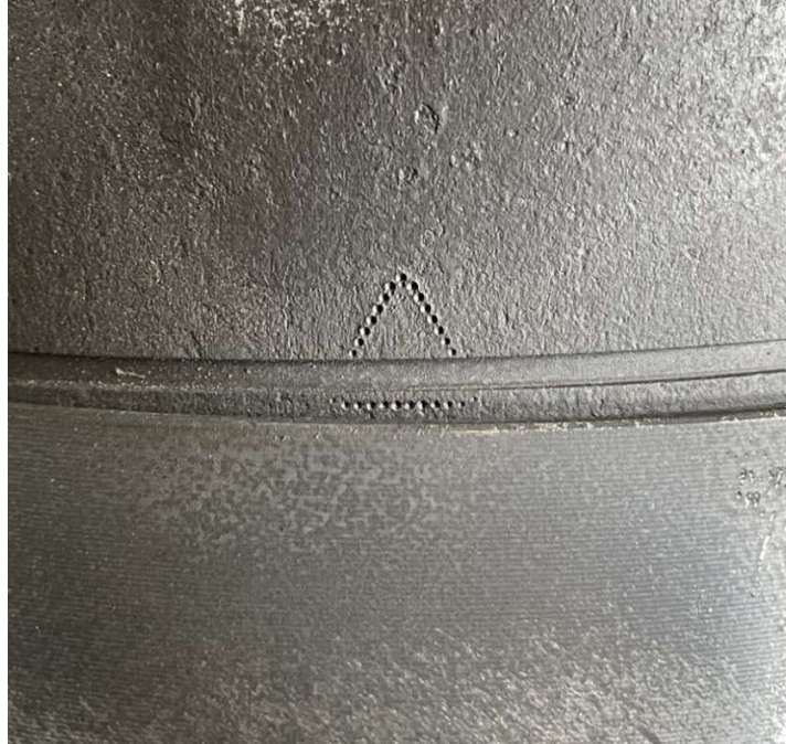
Figure 7: Example of Proper Triangle Stamp Position After Make-Up
