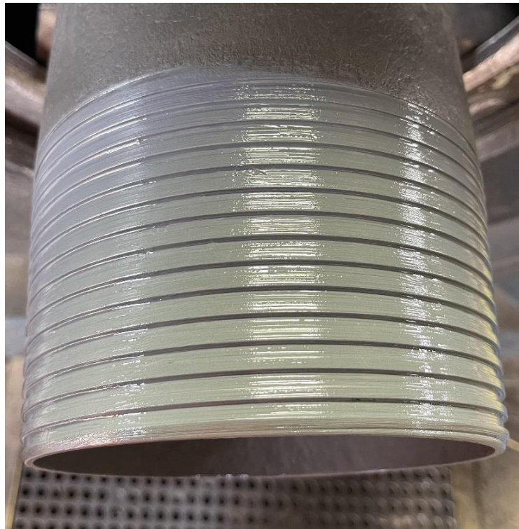
Figure 3: Example of Proper & Acceptable Thread Compound Application of the Pin Connection
