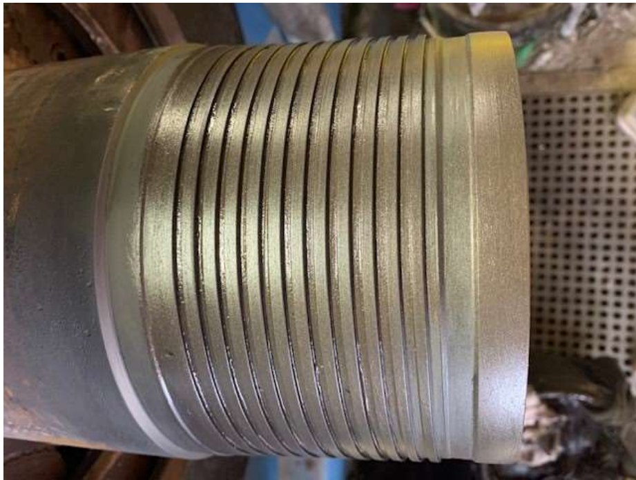
Figure 1: Correct way to apply thread compound.
