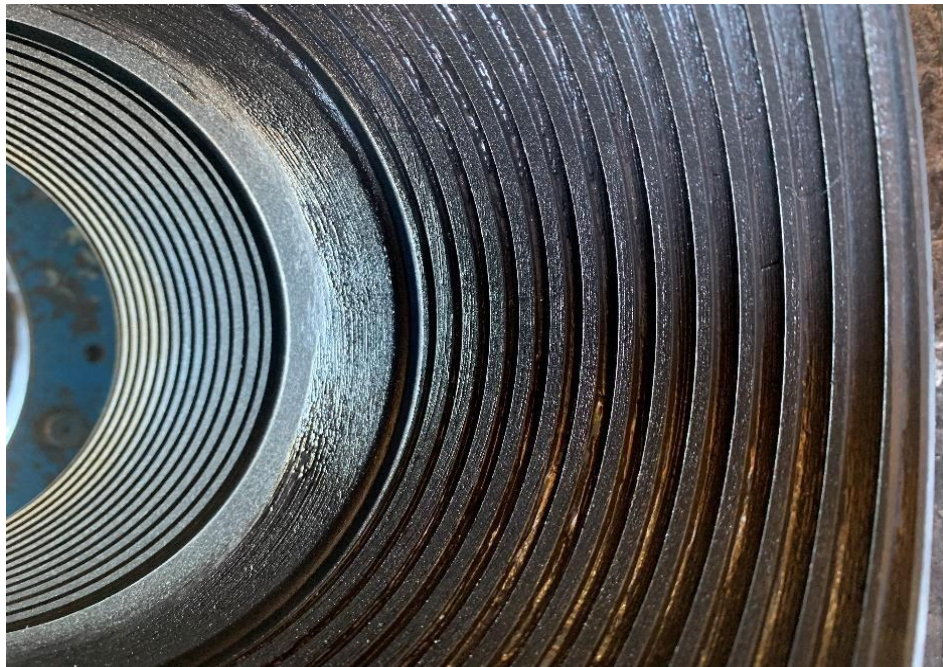
Figure 3: Example of Proper Thread Compound Application of the Box Connection
