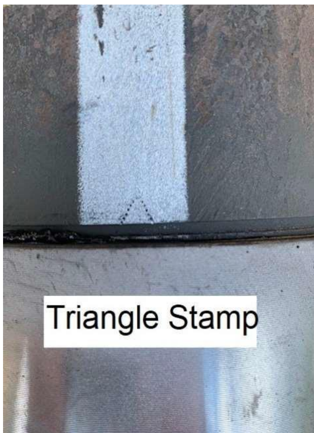
Figure 6: Example of Proper Triangle Stamp Position After Make-Up
