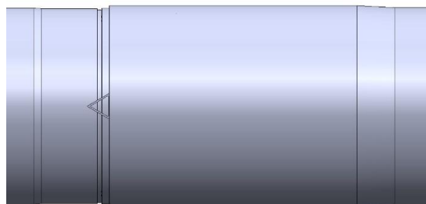
Figure 13: Triangle Stamp Location After Make-Up
