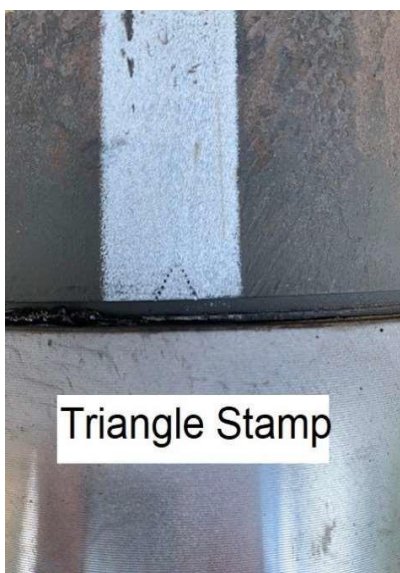
Figure 11: Example of Proper Triangle Stamp Position After Make-Up
