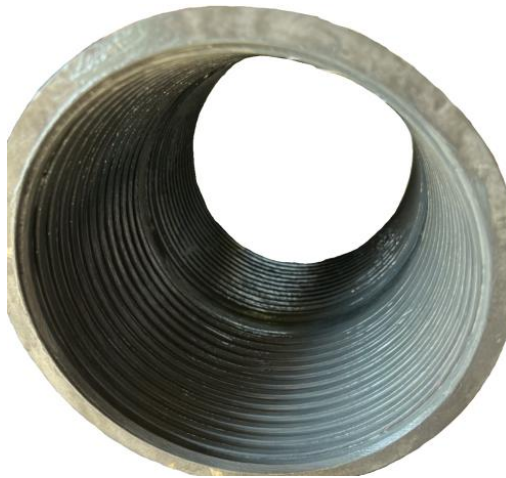
Figure 3: Example of Proper & Acceptable Thread Compound Application of the Box Connection
