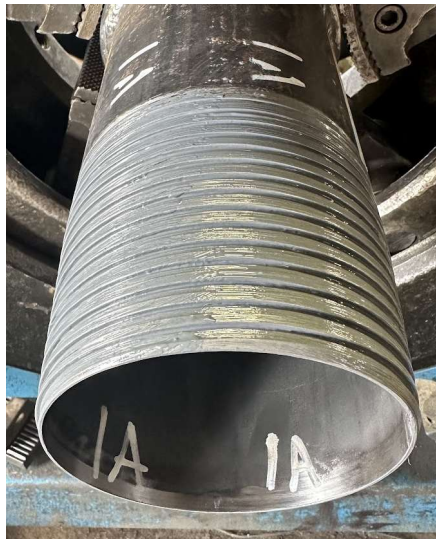
Figure 3: Example of Proper Thread Compound Application of the Pin Connection
