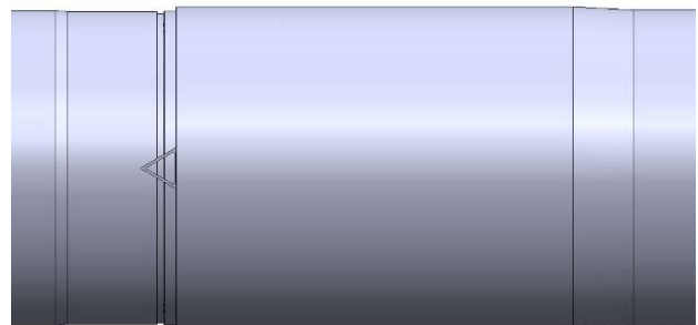
Figure 15: Triangle Stamp Location After Make-Up
