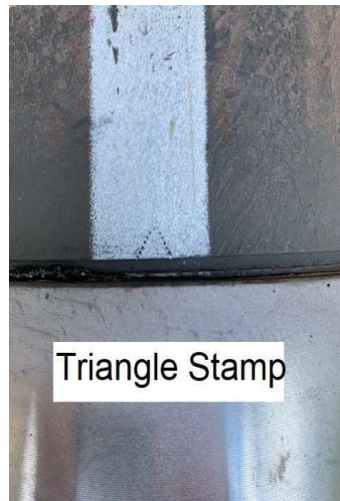
Figure 13: Example of Proper Triangle Stamp Position After Make-Up
