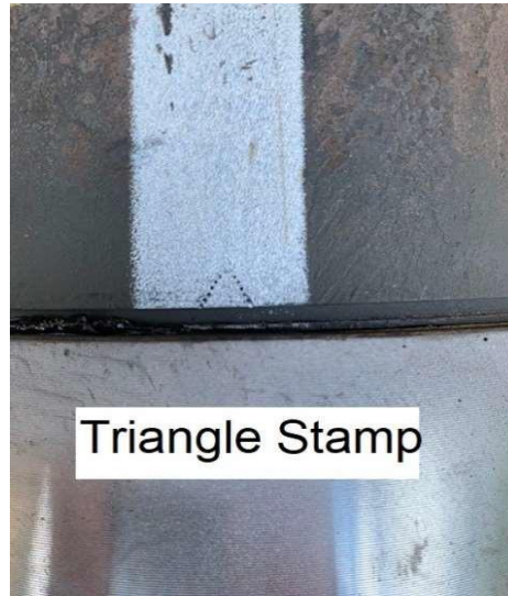
Figure 12: Example of Proper Triangle Stamp Position After Make-Up
