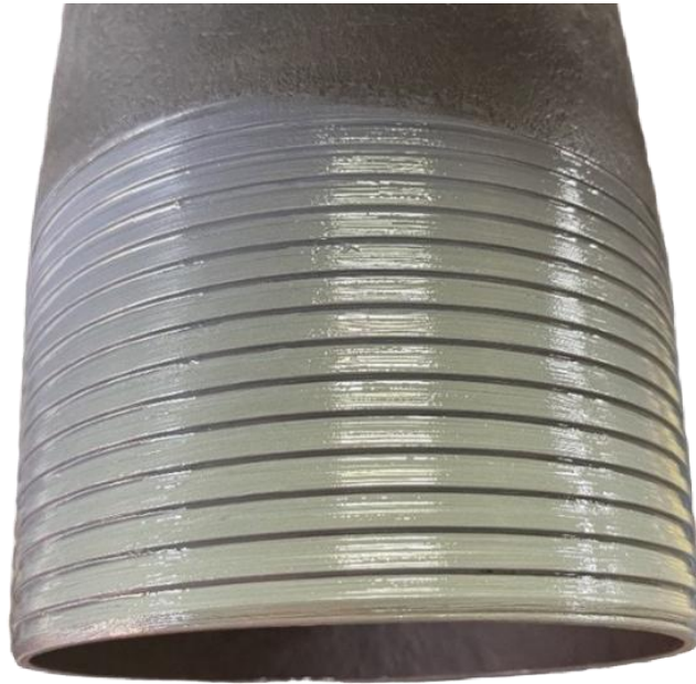
Figure 3: Example of Proper Thread Compound Application of the Pin Connection
