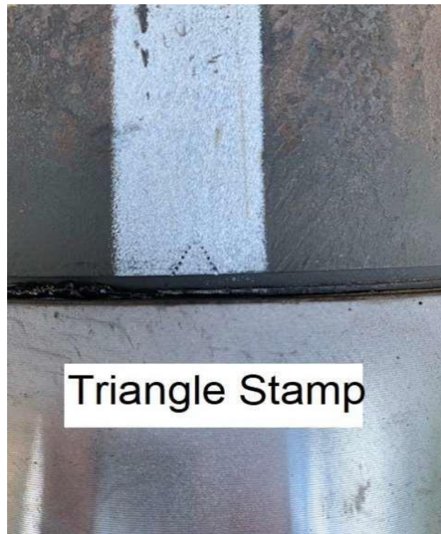
Figure 11: Example of Proper Triangle Stamp Position After Make-Up
