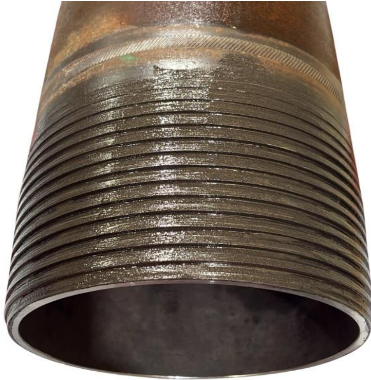
Figure 1: Proper Thread Compound Application Example
