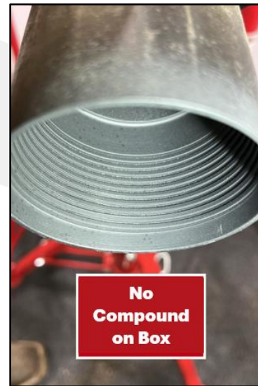
Figure 4 – Box Connection ( no compound)
