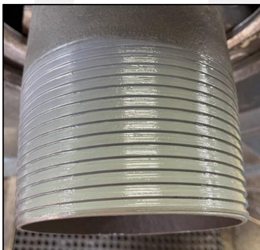
Figure 5 – Pin Connection Application
