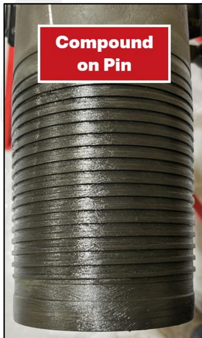
Figure 3 – Pin Connection Application
