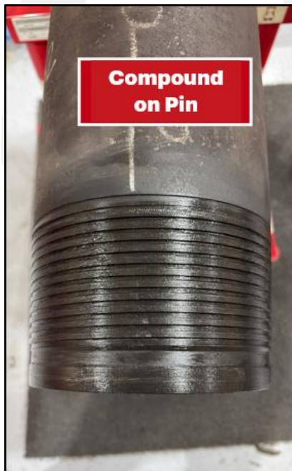
Figure 3 – Pin Connection application
