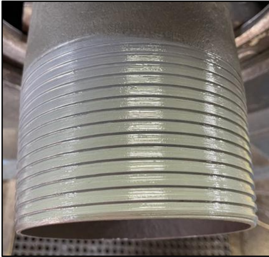
Figure 3 – Pin Connection Application
