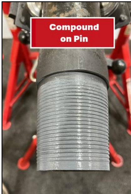
Figure 3 – Pin Connection Application
